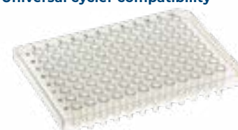
96-Well Semi-Skirted PCR Plate Straight edges
